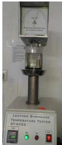
Gambar 1. Leather Shrinkage Temperature Tester GT-KC23
