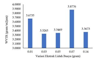
Gambar 6. Laju Transmisi Uap Air (Waver Vapor Transmission Rate) edible film variasi ekstrak lidah buaya
