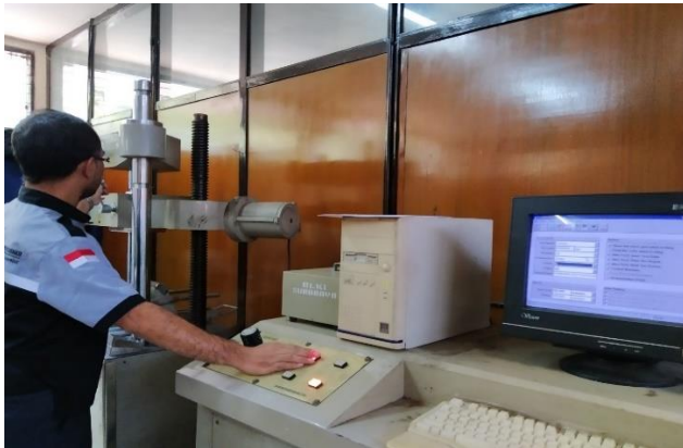
Figure 2. Bamboo tensile strength testing process.
