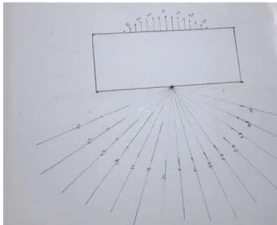
**Fig. 3.** Paper with inlet angle and exit angle reader indicators (inlet angle values are  $10^\circ$ ,  $20^\circ$ ,  $30^\circ$ ,  $40^\circ$ ,  $50^\circ$ , and  $60^\circ$ )
