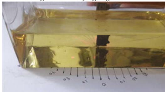
**Fig. 4.** Measurement of the refractive index of cooking oil using a refractometer that has been developed
