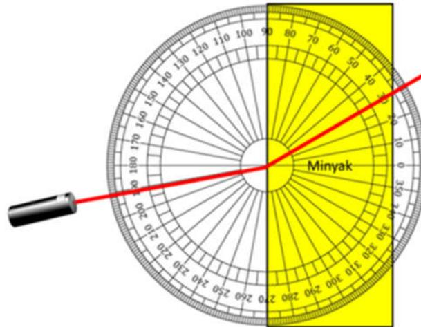
**Fig. 1.** The scheme for measuring the refractive index of cooking oil uses a container made of mica sheet by passing laser light through a container filled with the cooking oil sample to be tested
