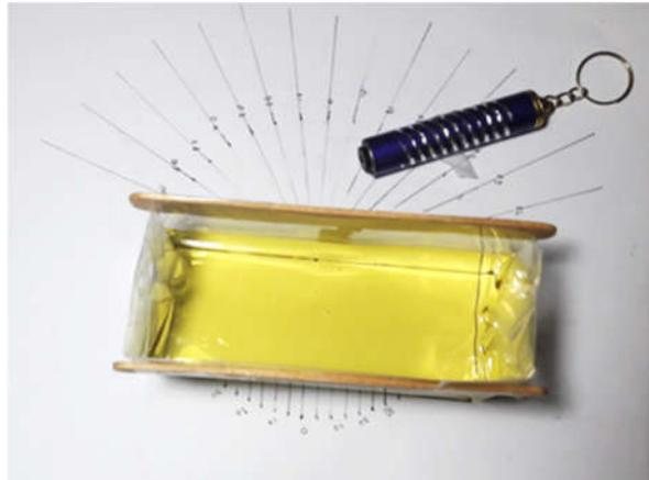
**Fig. 2.** Refractometer that has been developed
